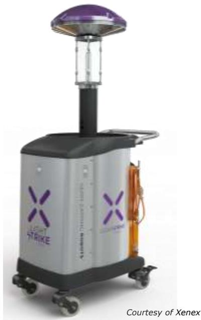
Beyond destroying microorganisms effectively, the high-intensity pulsed xenon UV light operates more quickly than other UV technologies. For example, the LightStrike robot runs an average of 5 minutes to deactivate C.diff spores compared to mercury bulbs requiring a 52-minute run time.
